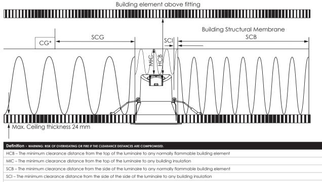
SCG – Side clearance to auxiliary equipment control gear (CG) (if supplied)
