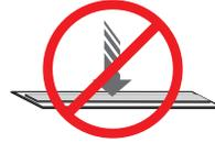
**DO NOT PUT EXCESSIVE PRESSURE ON SURFACE OF STRIP (GLASS/ACRYLIC PANES, ETC.)**
