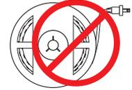
**DO NOT POWER STRIP LIGHT WHILE ON THE SPOOL OR TIGHTLY COILED.**
