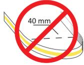
**DO NOT BEND LED STRIP LIGHT TO A DIAMETER LESS THAN 40MM**
