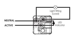
4.2 LED indicator off permanently, on momentarily (neutral required at switch) Load off permanently, on momentarily when press and hold
