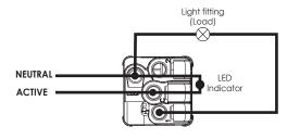
4.3 LED indicator permanently on, off when switch on (no neutral required)
