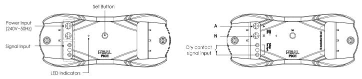
Functions - This product can be programmed to work either on "Latch" mode or "Pulse" mode, program must be operated with the PIXIE or PIXIE PLUS app.
