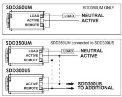
Note: An unlimited number of SDD300US can be connected to a SDD350UM. However, the total length of the remote wire (0.5 mm<sup>2</sup>) used to connect the SDD300US should not exceed 50 metres.
