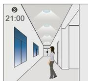
The light switches on at 100% when natural light is <30lux and there is movement detected.
