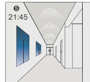
The light remains in 20% brightness dimming level at night if it can not sense any movement.
