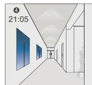
The light dims to stand-by level at 50% brightness after the 5min hold-time.
