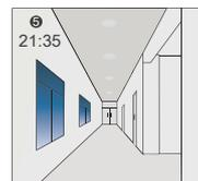
The light dims to off after 30min stand-by time if no movement is detected
