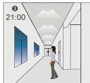
The light switches on at 100% brightness when natural light is <30lux and there is movement detected.
