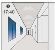
The light automatically turns on at 50% when natural light is <30lux even no any movement detected
