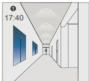
The light automatically turns on at 20% brightness when natural light is <30lux even no any movement detected.
