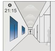
The light dims to stand-by level at 20% brightness after the 15min hold-time.
