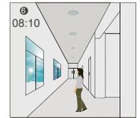
When the natural light level exceeds setpoint (>300lux), the light will turn off even if the space is occupied.
