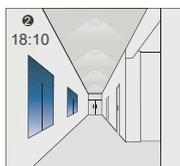
The light will turn off if it can not sense any movement after 30min.
