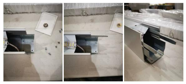
4. Repeat step 2 for the other \$9776, then connect two parts together, screw the rest two screws.
