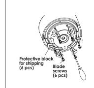
Remove the six blade screws from the bottom plate, and put it aside for use later.
